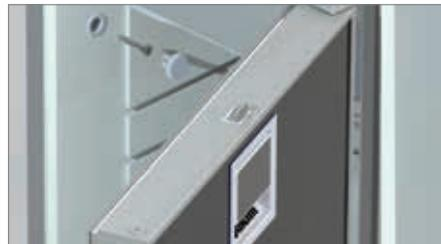
The new installation system allows an easy fixing of the cabinet directly from the interior of the fridge. The external flange is no longer necessary for the installation. An innovative internal bushing structure prevents the crushing of the insulated side wall.
